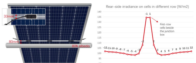
Figure 8: Typical rear-side light exposure of a bifacial half-cell module with a 1P horizontal single-axis tracker
